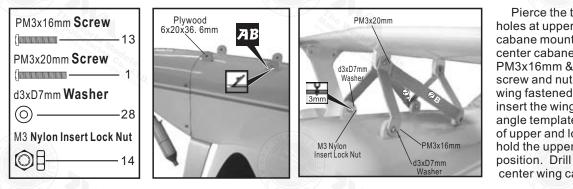
Pierce the two pre-drill holes at upper wing center cabane mount and fasten the center cabanes with PM3x16mm & PM3x20mm screw and nut. With the lower wing fastened to the fuselage, insert the wing incidence angle templates to both sides of upper and lower wing to hold the upper wing in position. Drill and fasten the center wing cabane with
