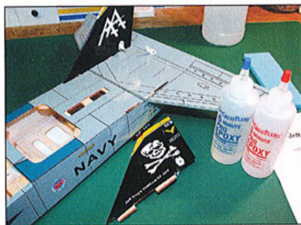
Self-aligning horizontal stabilizer and vertical fins are installed with 6-minute epoxy. Snaking the leads for the aileron servos is effortless thanks to two lengths of string that come factory installed in the F-14 TAMEcat's one-piece wing. Servo bays are factory cut.
