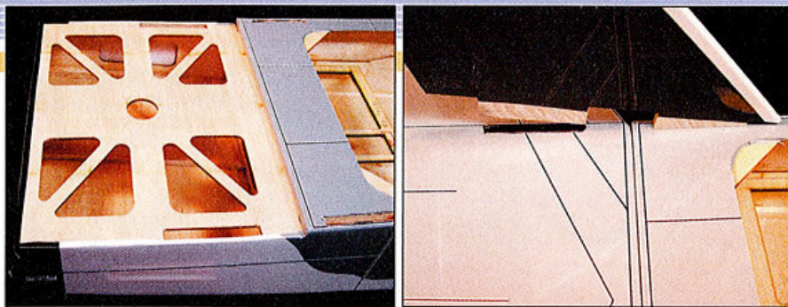
Tail saddle has ample gluing area for solid bond. Installing the stabilizer, then slipping the twin vertical fins into the slots assure perfect alignment with no measuring.
