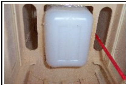
Fuel Tank Mounted
