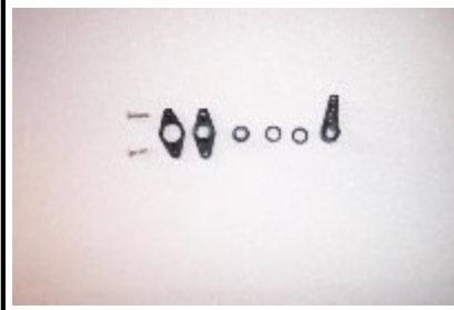
Elevator Linkage One Side
