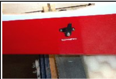
Elevator Control Horn
